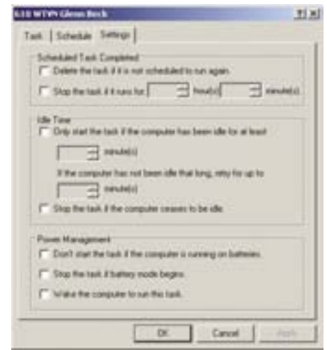
Example of the add schedule task wizard on the settings tab. I did not check any boxes because if the computer is running I want the radio to change.
