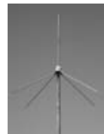
Quarter-wave Ground Plane with sloping radials. Radials 23 inches from antenna center. Vertical element 23 inches from insulator base.
