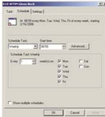
Example of the add schedule task wizard on the schedule tab. This is where the most of your scheduling happens.
