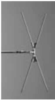
My "X" home brew antenna patterned after a dipole cluster antenna like the Scantenna but designed optimally for the VHF aircraft band. Fed with a TV type 300-75 Ohm transformer and then to RG-6. Diagonal dimension tip-to-tip is 47.5 inches.
