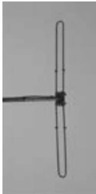
Folded dipole reworked from an Antennacraft FMSS Turnstile FM Antenna. Fed with a TV type 300-75 Ohm transformer and then to RG-6. Tip-to-tip dimension is 44.75 inches.
