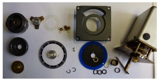
After putting the insert axis and the small ball in push the main axis back on the cog gear. If there was one of the cogwheel half disengaged, when the insert was pulled, you need to load the springs by pushing the last wheelpart 1 teeth in the good direction, not more, when more power is used on the back half of the cogwheel, is it possible to lose the small springs, they will jump out.
