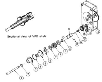
The exploded view of the gear displayed above is similar in build as the FT- series VFO gear. Clear to see is the construction of the balldrive. Pos 2, 3, 4, 5 and 6 are different in the FT gear.
