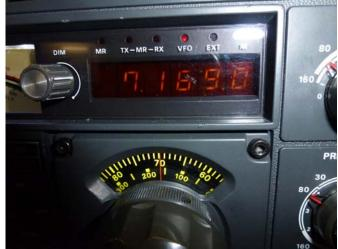
bandswitch and even see the S-meter wabbling when I connect an antenna. There is progress, but still no audio, but I can measure I.f. signals on the AF board. Changing the audioboard with the one of the 901 brings the audio back, and how! From the other board the TA-7205 audio IC is gone south, but my jobber had it in stock, so after changing a couple transistors and the chip, I have excellent audio now.
