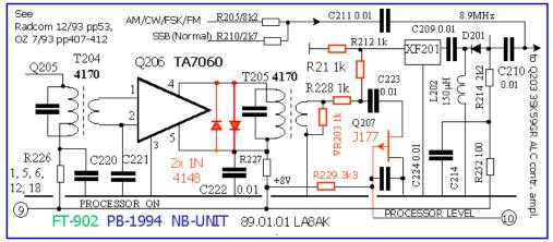
of speech, while perhaps very good for single tone transmission...... The LIMITER (Q206 TA7060P) was suspected, a pair of 1N4148 diodes were mounted in antiparalell across the output from this IC, and the RF CLIPPER functioned !! Just as easy it was to improve this. The same suspect circuit has been seen in some other FT-line transceivers.
